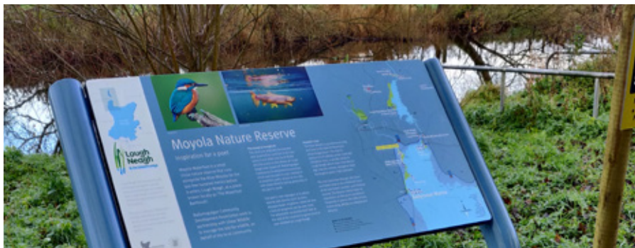
Low-level angled interpretation panel with clear knee space, adjacent to external route at Moyola Nature Reserve Riverside Walk
