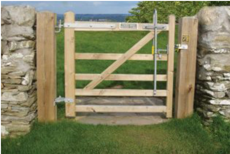
Aston Centrewire gate with easy open latch and 1700mm overall width; robust bottom rails make it suitable for mobility vehicles (Image courtesy of Centrewire)
